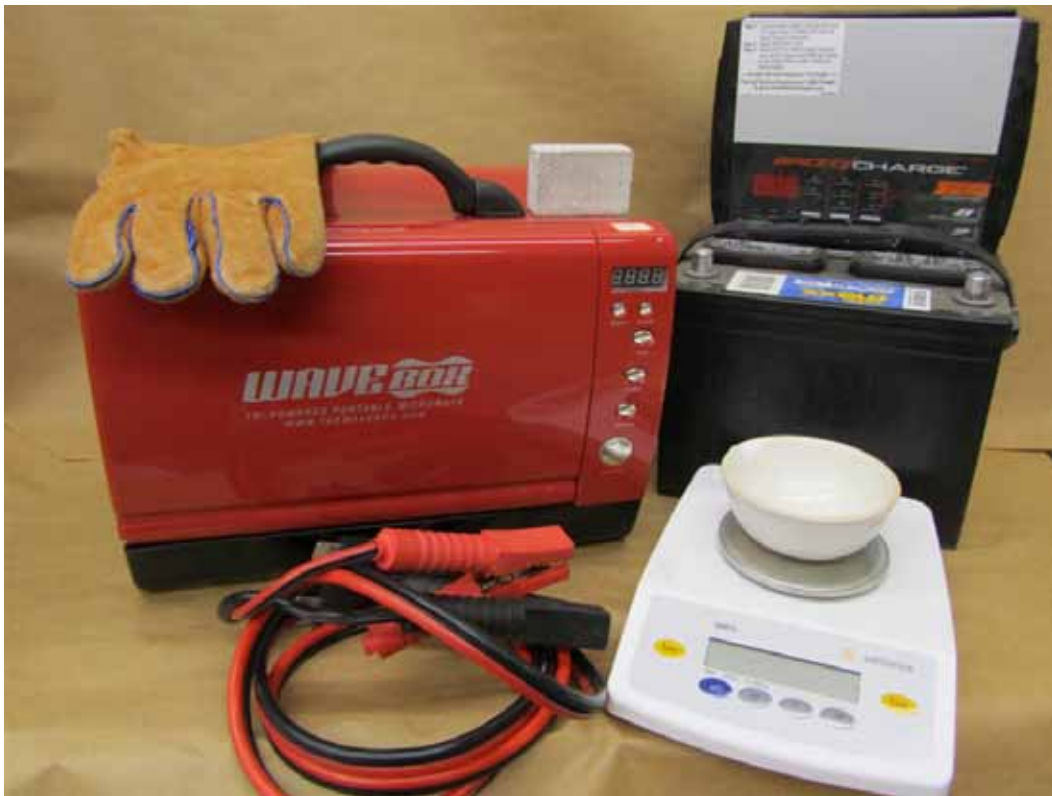
Figure 3. Variable wattage, 12-V powered WaveBox portable microwave oven.
