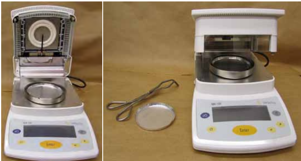
Figure 4. Sartorius model MA 150 1,200-g moisture analyzer.
