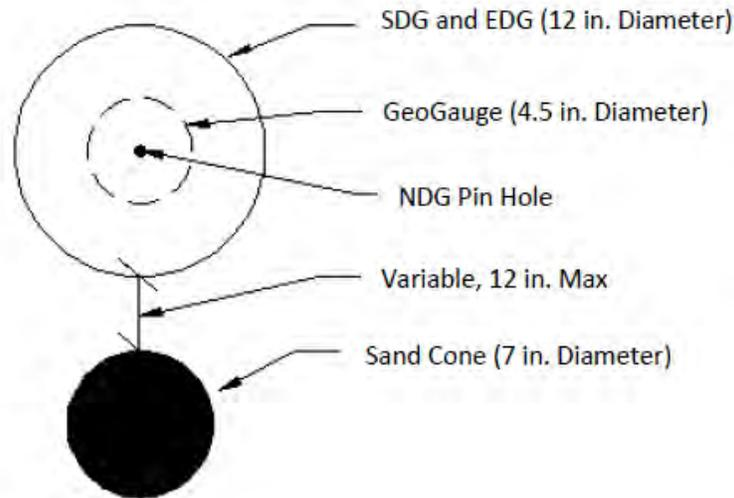
**Figure 16. Unbound Field Testing Pattern**
