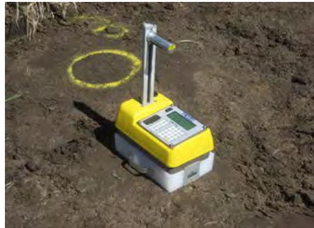
**Figure 15. Troxler 3440 Nuclear Density Gauge**
