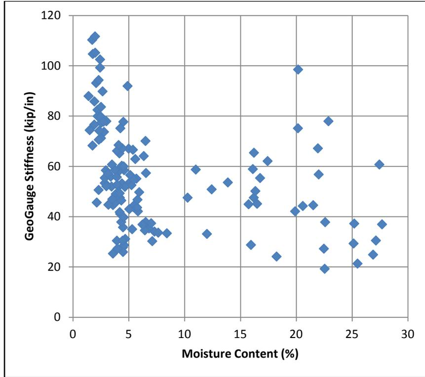
Figure 94. GeoGauge Stiffness vs. Oven Moisture Content
