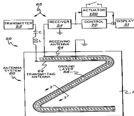
Figure 2. Operational and Receiver Diagrams for Troxler PaveTracker<sup>(5)</sup>
