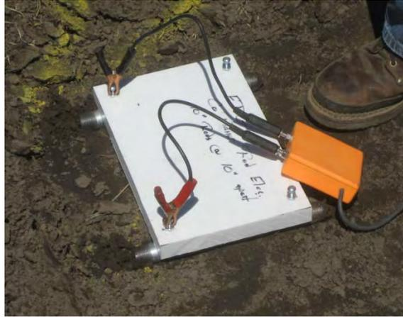
**Figure 81. EDG Plate Prototype Device**
