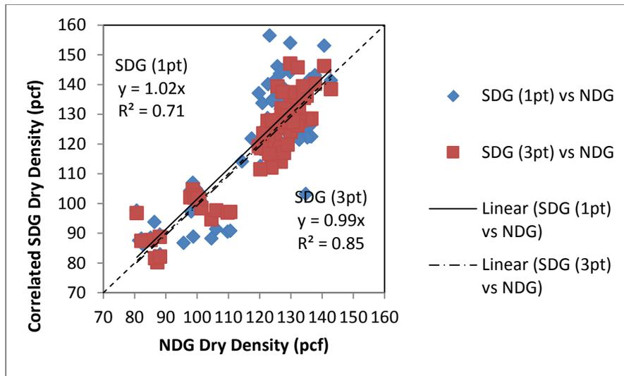
Figure 63. Dry Density Validation: SDG vs. NDG
