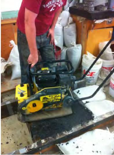
**Figure 14. Laboratory Compaction Using Vibratory Plate Compactor**
