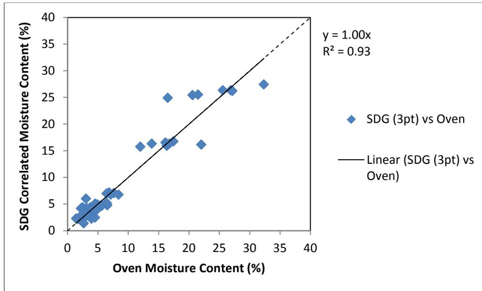
Figure 69. Moisture Content Validation: SDG (3 pt.) vs. Oven
