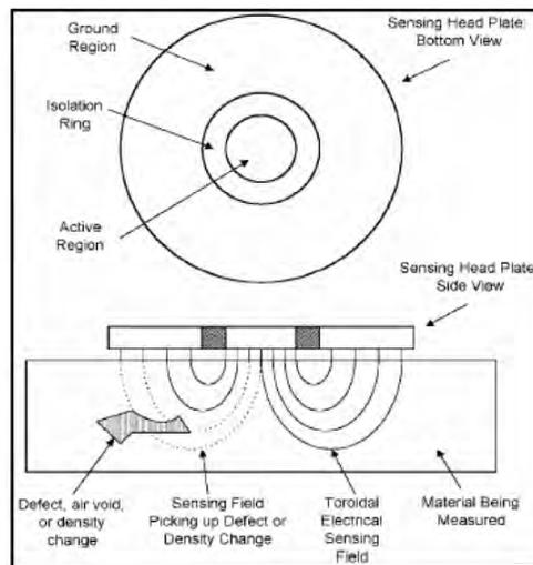
Figure 1. Operational and Receiver Diagrams for Trans Tech PQI<sup>(3)</sup>
