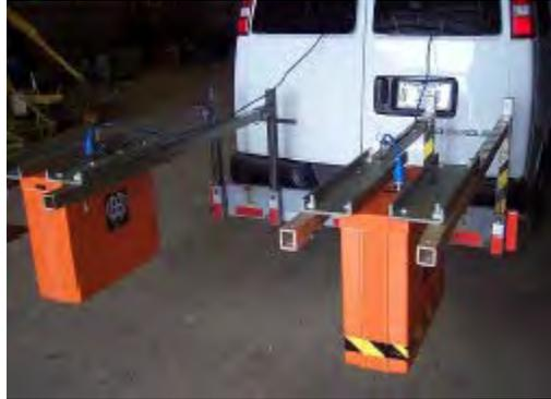
**Figure 5. Air Coupled GPR System<sup>(16)</sup>**
