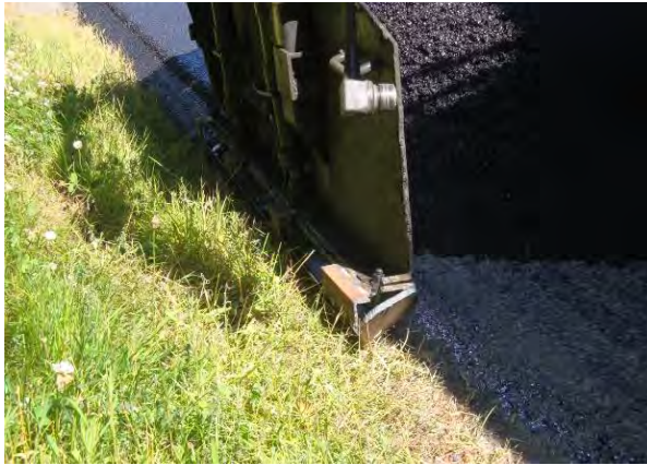
Figure 29. End view of TransTech pavement hardware without the roller.
