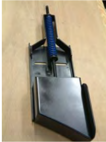
Figure 12. The Advant-Edge™ creates a tapered 30° safety edge along the shoulder of the road.
