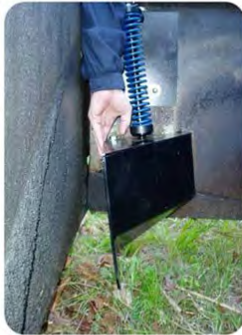
Figure 9. Troxler SafeTSlope™ Edge Smoother.
