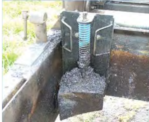
Figure 1. Pavement edge “shoe” bolted to paving machine screed (FHWA).
