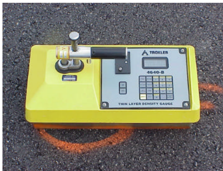
Figure 2. Troxler Model 4640-B Nuclear Density Gauge.
