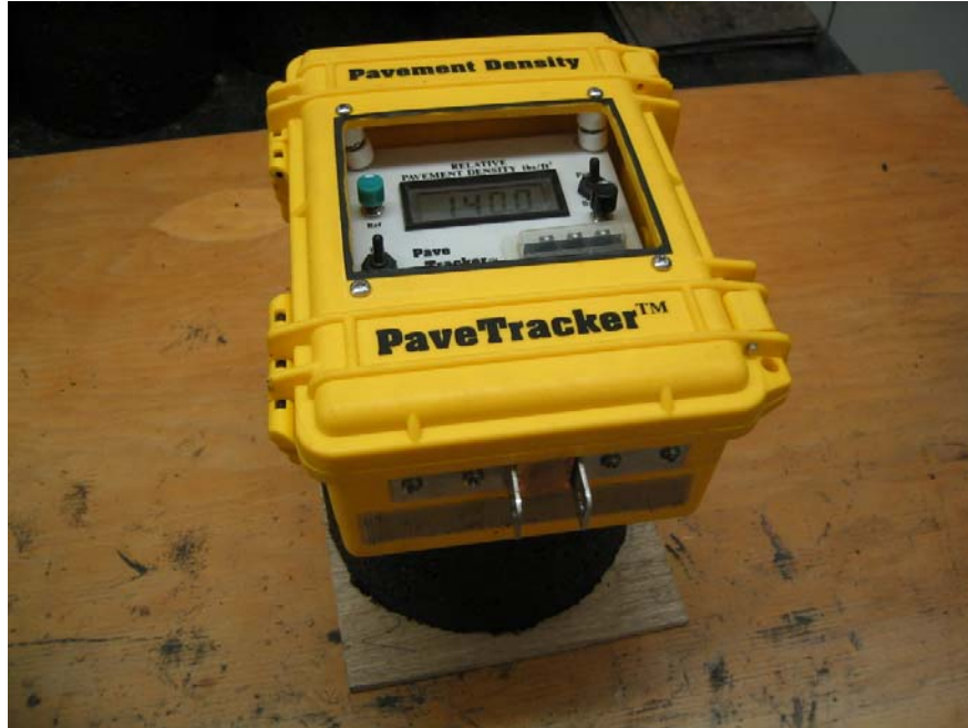
Figure 5. Pavetracker™ on Superpave Gyrotory Sample
