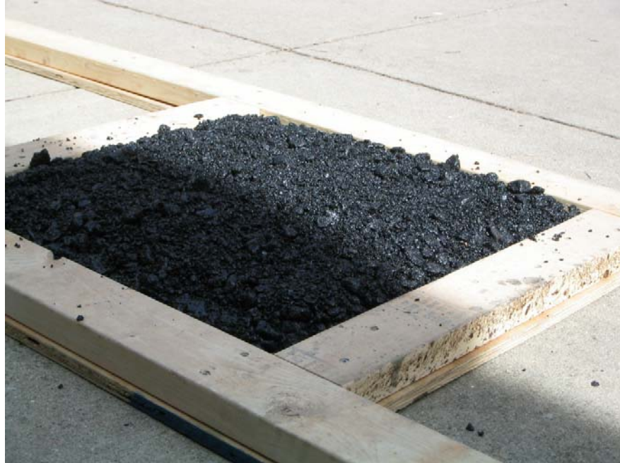
Figure 2. Timber Wood Compaction Mold with Loose Mixes Inside
