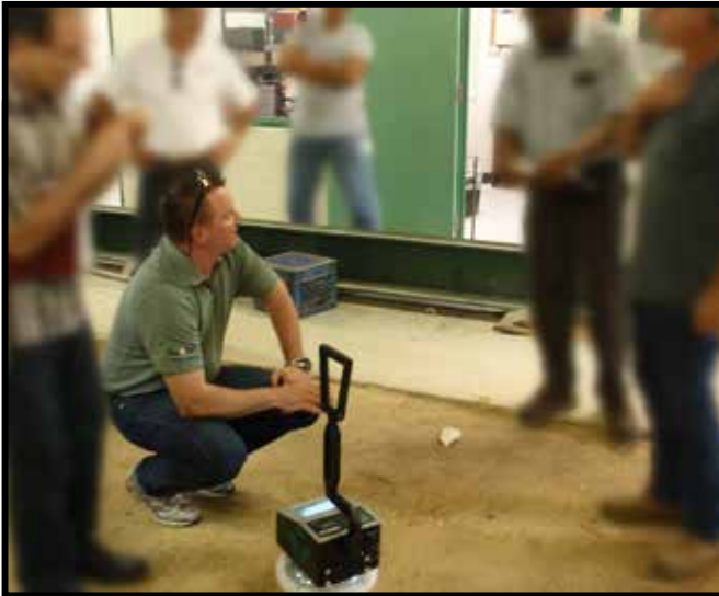
Atlantic Supply and TransTech Systems demonstrate usage of the SDG 200 Non-Nuclear Soil Density Gauge to the Florida DOT
