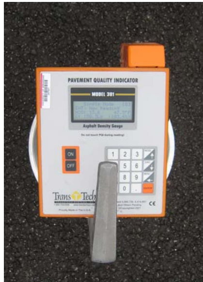
Figure 4. Pavement Quality Indicator™ (PQI) Model 301
