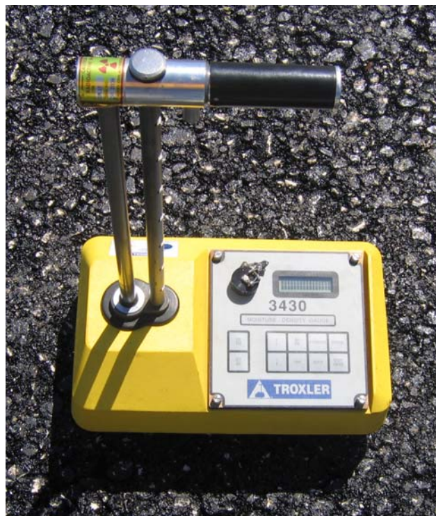
Figure 2. Troxler Model 3430 Nuclear Gauge
