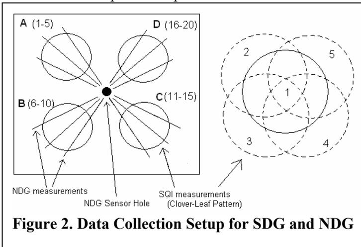
CPN MC3 Portaprobe with a 12-inch rod and with a current factory calibration, following the pattern shown in Figure 2, after one, two, four and eight compactor passes. In Figure 2, the four circles, labeled A, B, C and D, represent the centers of the SDG measurements and the three lines over the SDG circles represent the
