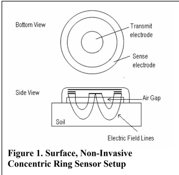
**Figure 1. Surface, Non-Invasive Concentric Ring Sensor Setup**
